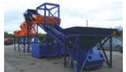
Conveyor with Overband Magnet, Baler, Vibro Feeder & ECS Unit
